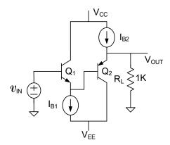
Problem 6 Consider the two amplifier circuit shown below where  $V_{DD}=5V$ ,  $I_{B1}=5\mu A$ ,  $I_{B2}=10\mu A$ , and  $R_L=5K$ . Assume the transistors are identically sized with W=10 $\mu$  and L=2 $\mu$ .
